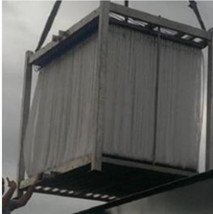
Membrane Aerated Biofilm Reactor
