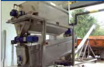
DSP Screw Press Model 3012, NY WWTP
