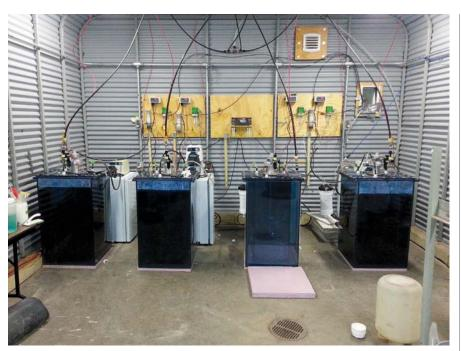
Figure 3. Pilot Digesters Used in the MCES Research Program
