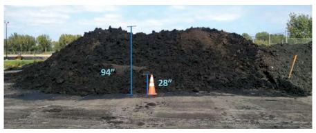
Figure 7. Biosolids Stockpiled in a Manner to Reduce the Impact of Rain
