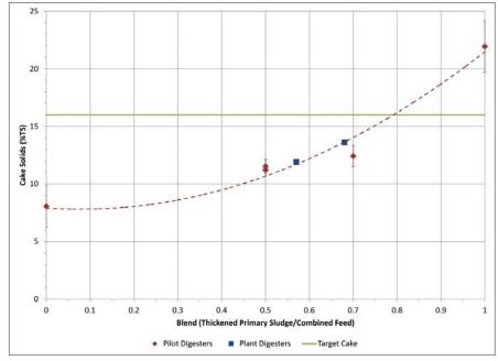
Figure 4. Full-Scale and Pilot-Scale Dewatering and Blend of Feed Sludge
