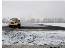
Figure 6. Biosolids Storage Use to Enhance Drying – Solids Spreading
