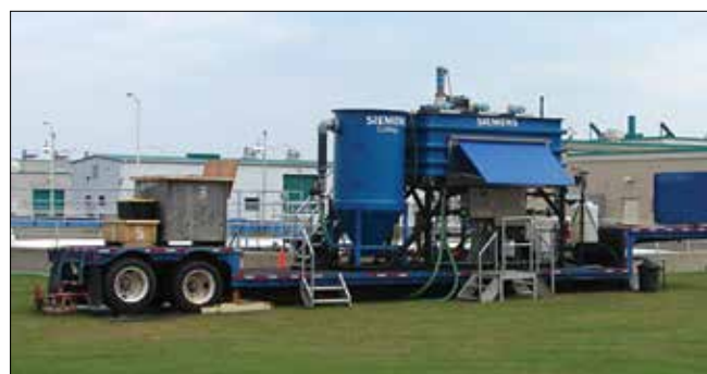
Figure 1 CoMag ® pilot trailer (50 gpm) on site at the Fond du Lac WPCP.
