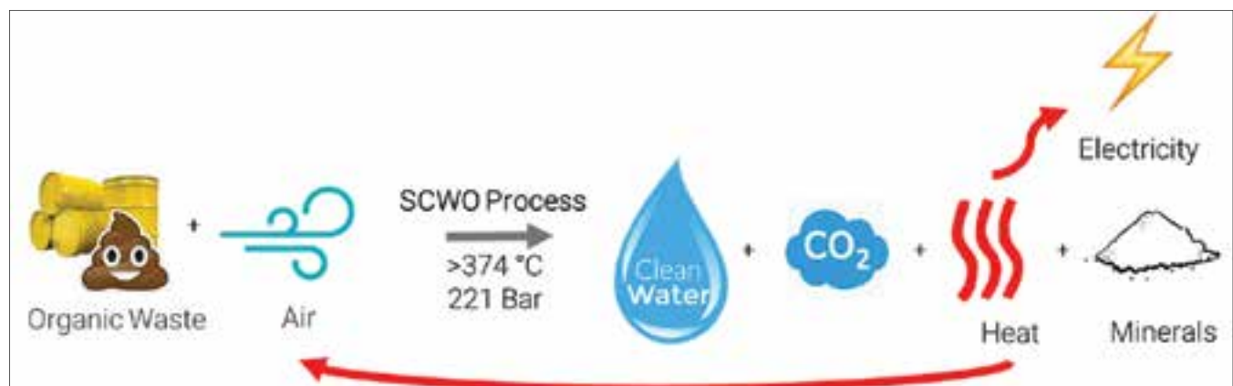
Figure 1. Supercritical Water Oxidation (SCWO) Reaction Equation
