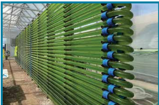
The mercury trial conducted in 2019 aimed to use a CLEARAS ABNR system to remove mercury waste from wastewater.
