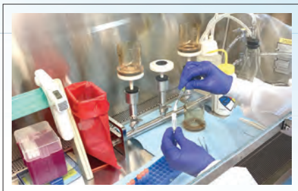
After the wastewater is concentrated by filtration, Dr. Kayley Janssen rolls up the filter and places it in a tube filled with beads to be homogenized.
