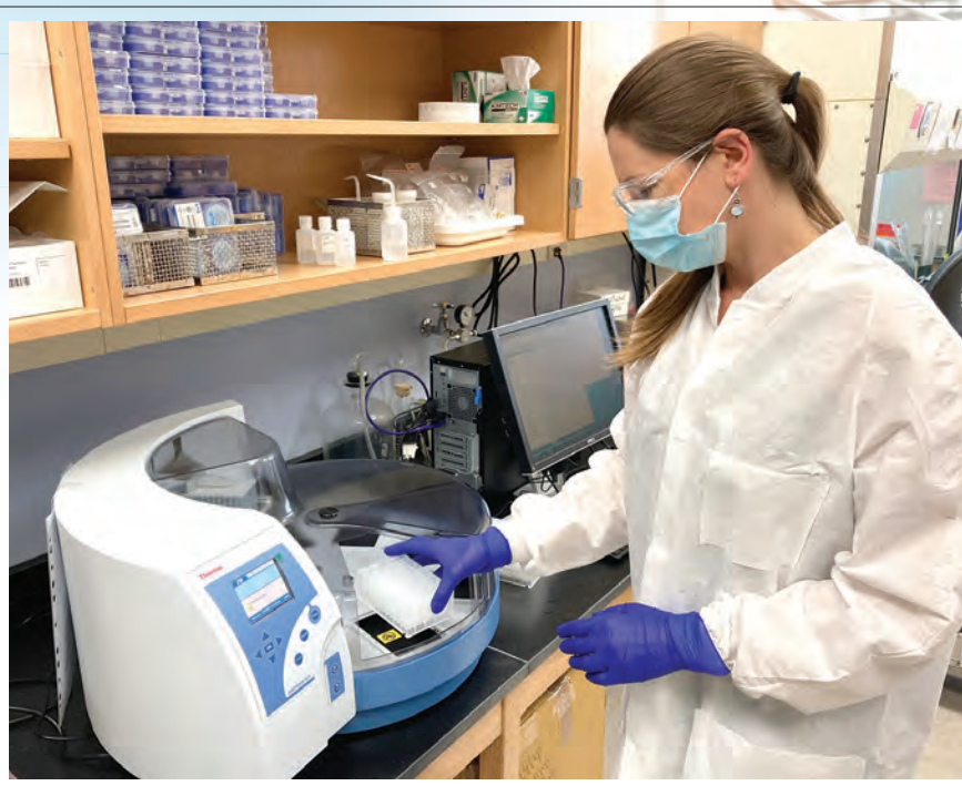
Dr. Dagmara Antkiewicz sets up instrumentation with the concentrated and homogenized wastewater sample for the extraction of genetic material to test for the presence of SARS-CoV-2.
