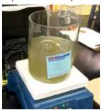
FIGURE 2 – Jar Testing Experimental Setup (Stock Solution Adjacent to Sample)
