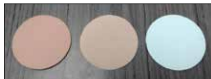
\text{Fe}_2\text{O}_3/\text{TiO}_2 hybrid nanowire membrane with different \text{Fe}_2\text{O}_3 concentration
