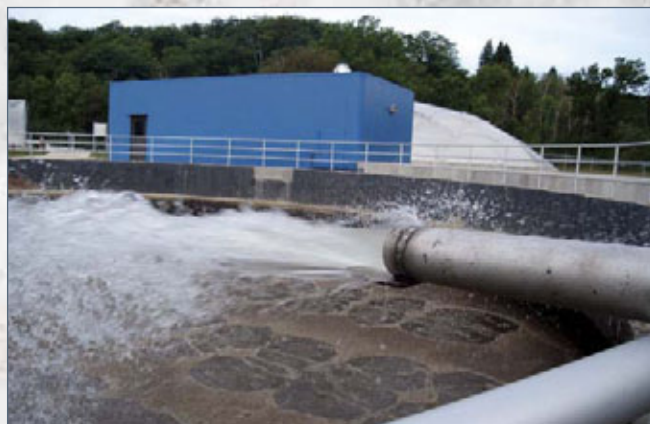
Testing of foam suppression nozzle with bottom flat plate discharge at WAS storage tank. Note evidence of brown scummy foam at tank surface.
