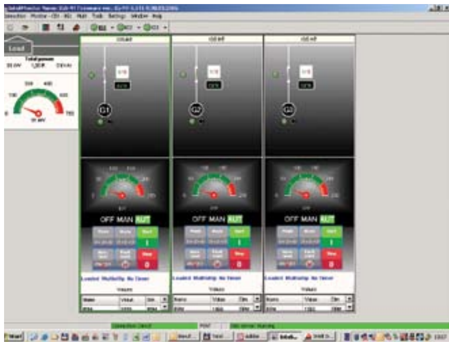
Remote PC monitoring for multiple gen-sets (Courtesy ComAp, spol. s r.o.)
