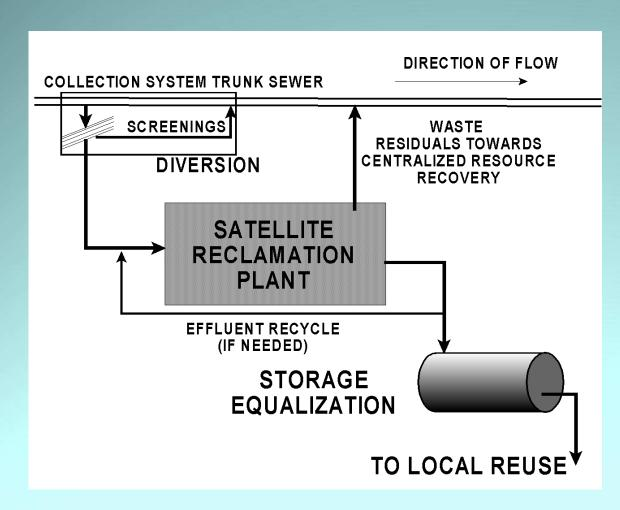
Package and small high efficiency treatment units can be installed to provide locally water for:
