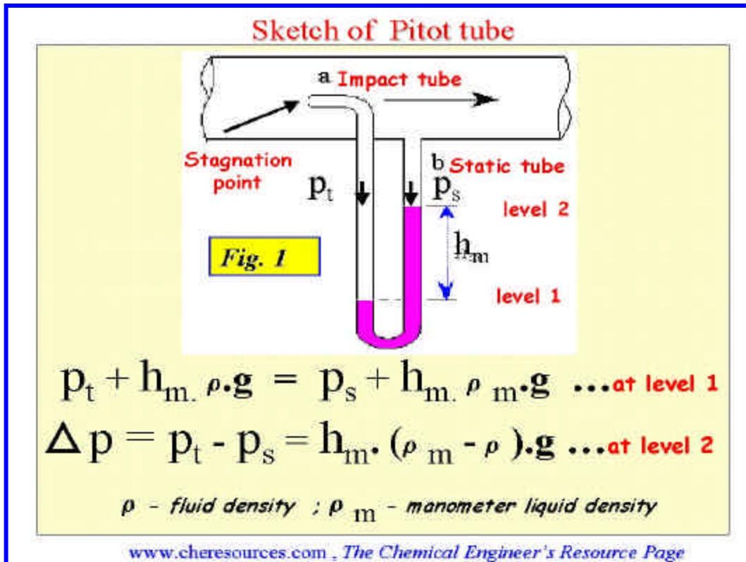
**Figure 1: A Simple Sketch of a Pilot Tube**
