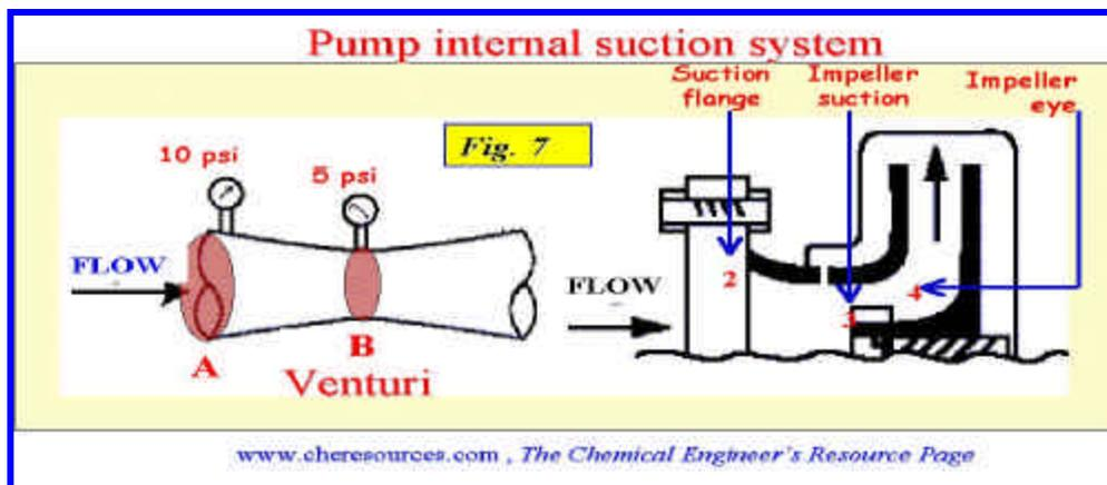
**Figure 7: Pump Internal Suction System**
