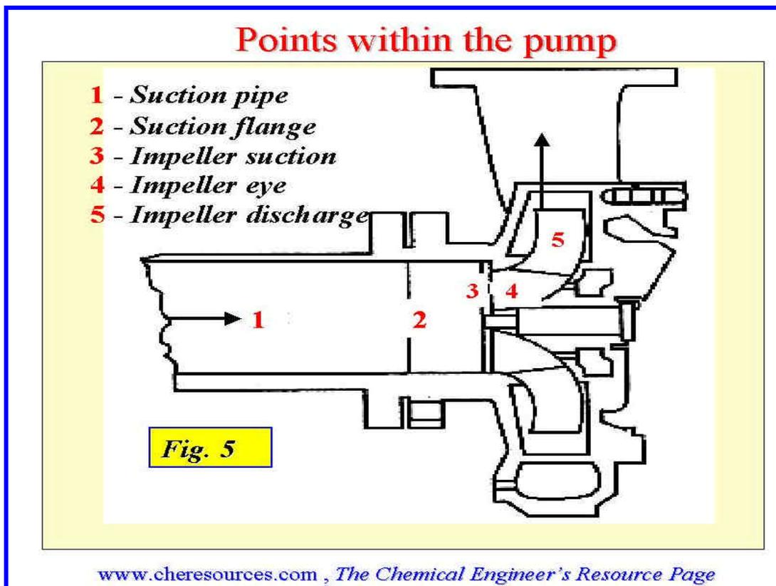
**Figure 5: Internal Pump Locations**
