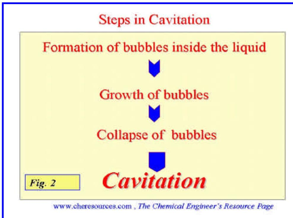
**Figure 2: Phenomenon of Cavitation**
