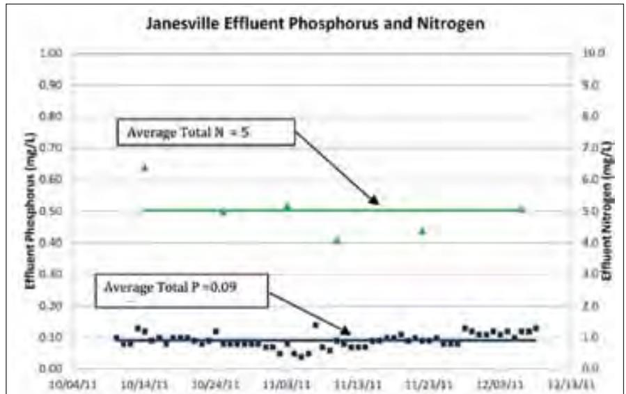
Figure 1: Janesville Nutrient Removal Performance when receiving ethanol plant wastewater
